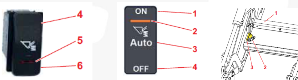
Possible variants for activating the ComfortDrive (1. electric, 2. electric depending on the speed, 3. mechanical)
